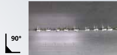
Corner spot welding thickness 0,6 mm
